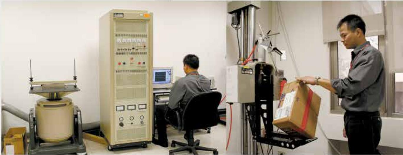
MEAN WELL has a complete quality management system. To ensure product quality, 100% burn-in test, function test and pressure test have been applied in manufacturing process, while the MIL-105E sampling method used in IQC, PCBQC (semi-finished products testing) and FQC phases. In the R&D stage, MEAN WELL quality engineers customize the “Test Plan” for each product, to complete the verifications of DFMEA, DVT/DQT, ORT, EMC, drop test, vibration test, thermal shock test, and reliability test.
